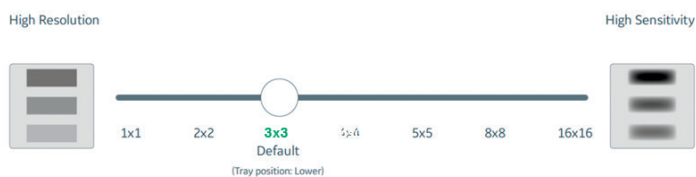
Fig 11. The CCD detector of ImageQuant 800 imager allows for on-chip binning. Default settings (5×5 for upper and 3×3 for lower tray position in chemiluminescence mode) can easily be changed using the slider. Low binning levels improve the resolution and high binning leads to shorter exposure times.
